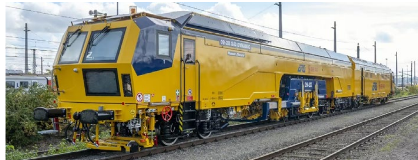
Linjski stroj za smerno in višinsko uravnavanje tira. Vir: https://www.plassertheurer.com/en/machine/track-tamping-machines/O9-x-series/O9-2x-sd-l-dynamic
